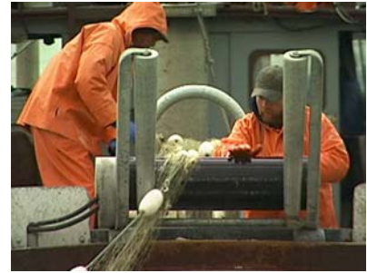
Gill net spooling out from the stern of drift fishing boat. Rapid spool out and retrieval is key to a profitable boat.
