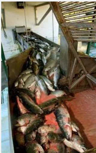
Salmon move along a conveyor that brings the fish into the Englewood Packing Co. in Port, McNeil, British Columbia. The salmon have their gills cut and are electrically stunned as they begin to move along the conveyor. The chilled water becomes foamy and turns pink as oxygen is released from the blood of the fish after their gills are cut.
