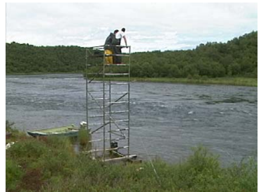
Counting Towers used by Fish & Game. The salmon are counted with a low-tech technique. The fish counter wears polarized sunglasses to better see through the water and the salmon are visually counted. Long hand math, multiplying the number of salmon seen in 10 minutes on both banks, by the number ‘6’ finish the job.
