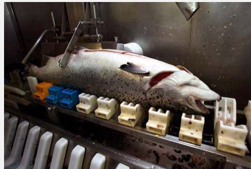
Salmon on a conveyor is cleaned and gutted by a machine at the Englewood Packing processing plant on Vancouver Island.
